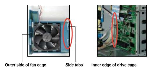
3. Push the outer edge of the fan cage sideways to fit it to the drive cage. You hear a click when the fan cage correctly fits in place.
